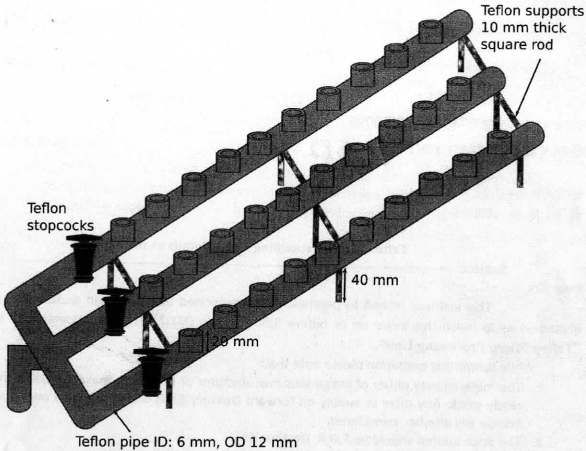
All joints in the above apparatus should be leak proof against 20 M hydrochloric acid flow.
